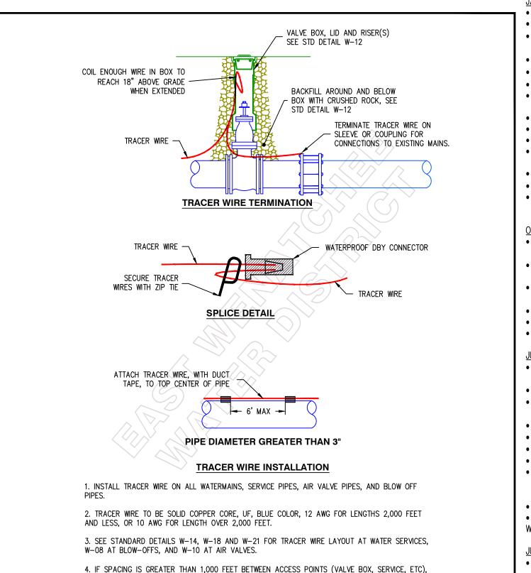
PROVIDE A VALVE BOX FOR TERMINATION AS SHOWN ON THIS DETAIL.
